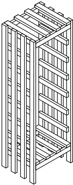
2. Nail only the bottom shelf to the side rail. Leave the top shelf to keep the spacing.
