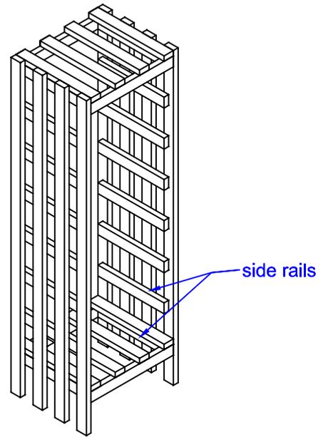
3. Keep adding shelves from the bottom up and nailing them on. Securing the top last.
